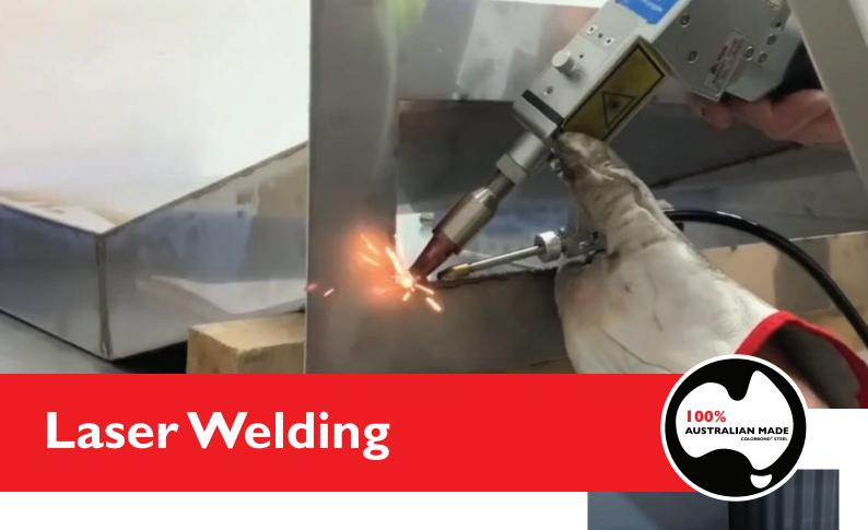
Laser welding is ideal for high-precision, high-speed applications, especially for thin metals. Roofing & Sheetmetal Centre can laser weld sheet metals like stainless steel, aluminium and galvanised steel in gauges between 1.2mm to 2mm.
